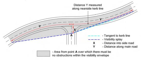
Visibility splays must be checked at every junction. The visibility splay requirements vary depending on the category and design speed of the **main** road.
