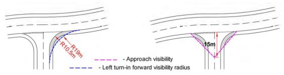
The approach visibility should be checked for local distributor and non-residential roads and connecting streets. It is measured 15m back from the give way line along the centreline of the side
