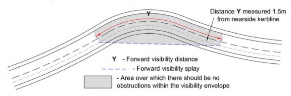
The above diagram demonstrates the method for constructing a single forward visibility splay. The forward visibility distance, **Y**, is determined by the category and design speed of the road. The minimum forward visibility values set out in the table below should be used:
