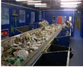
On the first conveyor an initial hand sort is carried out to remove any large recyclable items such as card and contamination (non-recyclable items) such as crisp packets and plastic bags.
