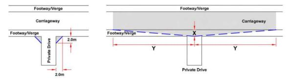
The **X** distance should be 2.0m for private drives and 2.4m for shared drives. The **Y** distance is the minimum forward visibility distance of the main road. Pedestrian visibility to back of footway to be  $2.0m \times 2.0m$  on both sides.
