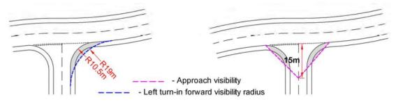
The approach visibility should be checked for local distributor and non-residential roads and connecting streets. It is measured 15m back from the give way line along the centreline of the side road. Drivers should be able to clearly see the layout of the junction on approach to the main road. The left turn-in forward visibility radius should be checked at every junction. The radius should be drawn tangential to the side road and main road kerblines.
