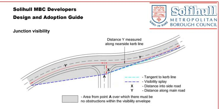
Visibility splays must be checked at every junction. The visibility splay requirements vary depending on the category and design speed of the **main** road.
