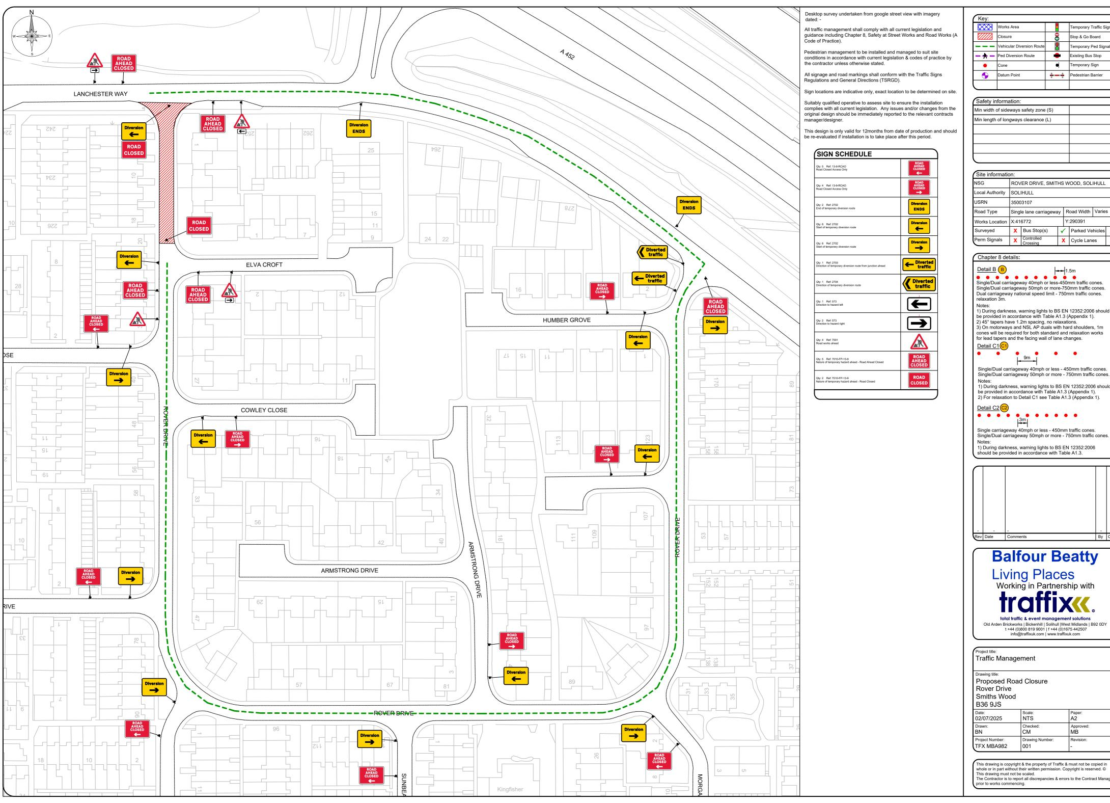
Temporary Traffic Signa Stop & Go Board Temporary Ped Signal Existing Bus Stop Temporary Sign
